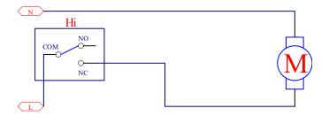
Current less than 2A can be directly connected to the load
