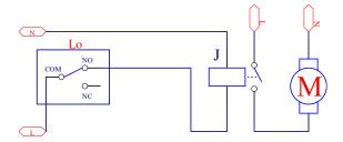
Connect low relay conductance values or resistance value decline to the setting value can automatically close dosing device
