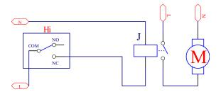
Connect high relay conductance values or resistance value rises to the setting value can automatically open dosing device
