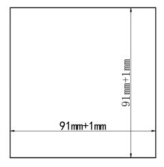
2. The instrument rear is inserted from opening front, two locking assembly and a locking.
