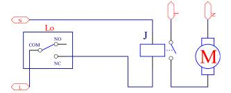
Connect low relay conductance values or resistance value decline to the setting value can automatically open dosing device
